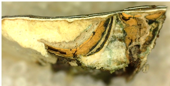
Example of a thick section of paint, where many layers and fillers/putties are overlapping. Areas like this will create confusion in analysis and identification.
