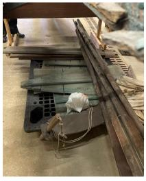
The mid-keel and immediate boards are rotten due to many years of storage in a damp location in Chicago. The rest of the boat is sound including deck boards, seats, rodder, oars and sale.
